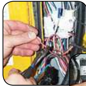
Clip the terminal pin off the removed wire. . .
