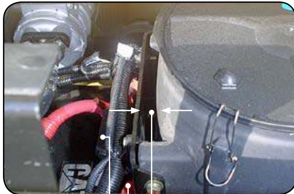
Shunt Assembly Plastic base will be replaced and re-mounted with through-bolts.
