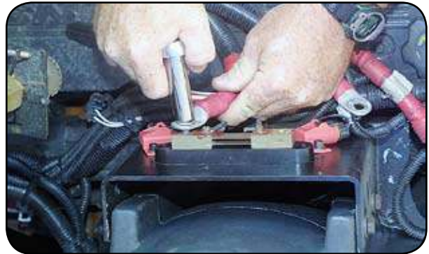
2 Small Signal Lead Screws Torque: 25-30 in lb.
