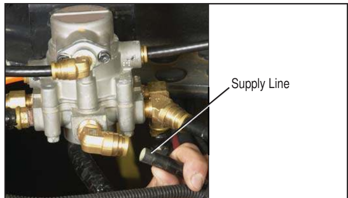
Figure 3 - DISCONNECTING THE SUPPLY LINE
