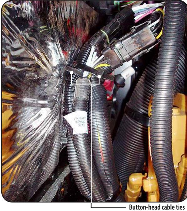
7.3 Inspect the battery cables for any evidence of contact with the rear of the engine, chaffing, or other damage. (Some harnesses may be attached to the engine lifting eye; those are not battery cables.)
